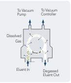
Dissolved gases are actively removed from a flowing liquid stream by vacuum via the Systec AF® membrane.
