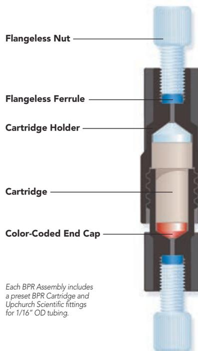
Each BPR Assembly includes a preset BPR Cartridge and Upchurch Scientific fittings for 1/16" OD tubing.
